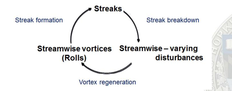
Rolls/streaks are critical to transition and turbulence
