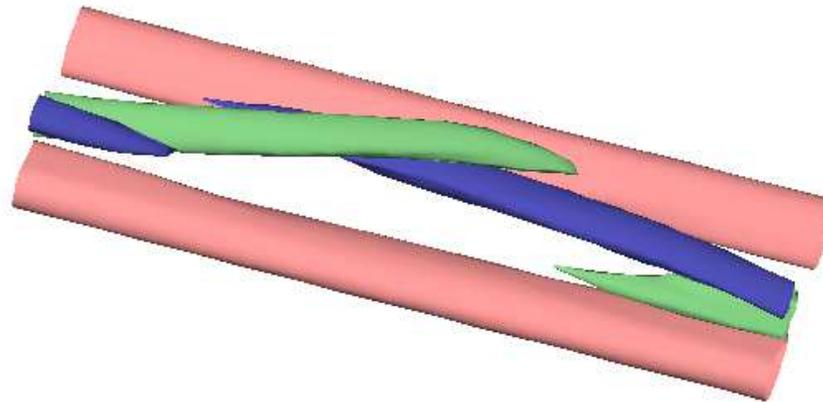
TW2-1: exact traveling wave of channel flow
