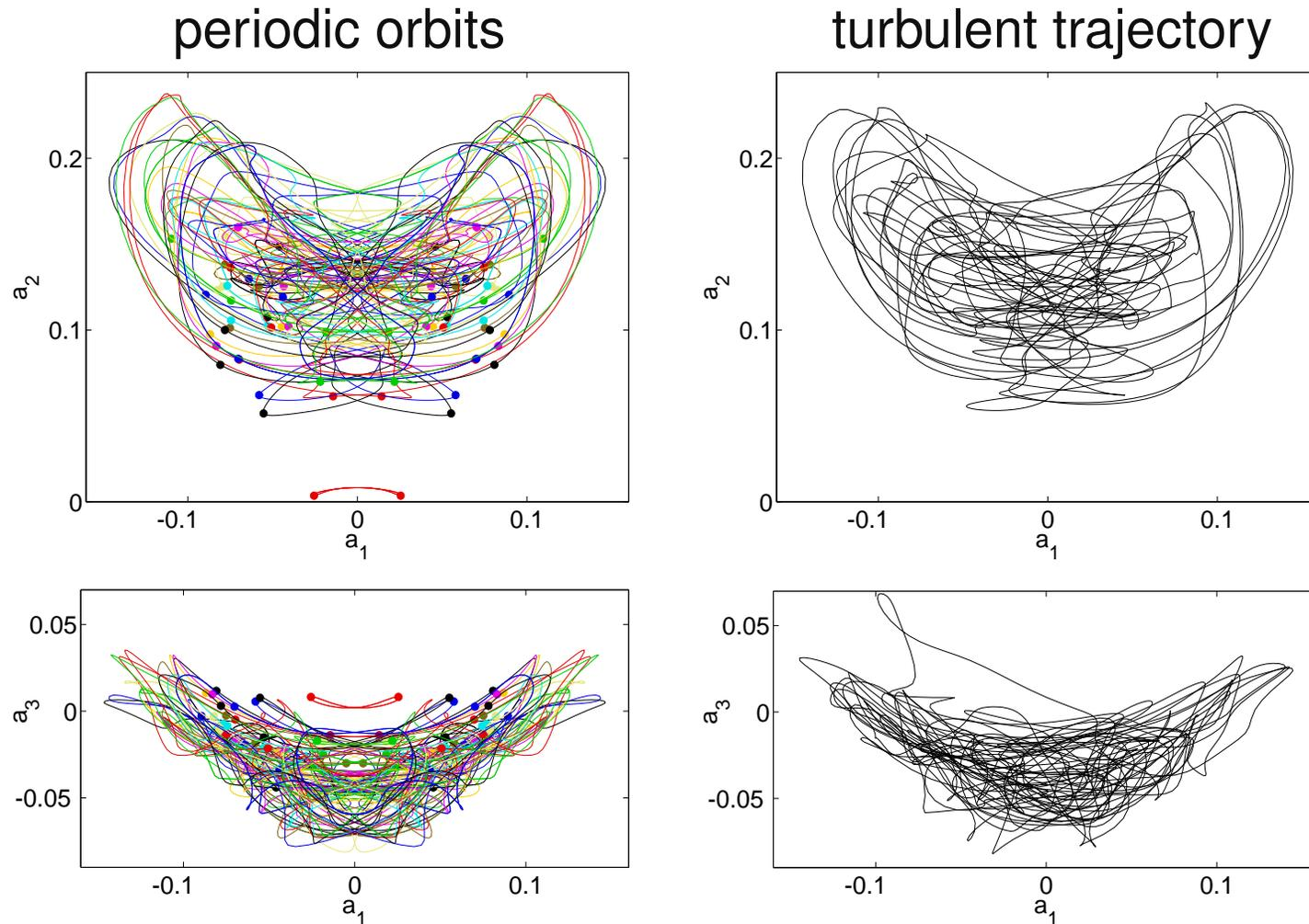
$10^5$ -d DNS states  $\mathbf{u}$  projected onto principal axes of a periodic orbit.
