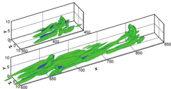
FIG. 2. (Color online) Snapshots of the streamwise component of the perturbation (darker surfaces, blue online, for  $u \cdot \nabla u$ ) and of the Q-criterion (lighter surfaces, green online) at  $t = 300$  and  $t = 700$  (top and bottom, respectively) obtained by the DNS initialized with the nonlinear optimal perturbation with  $E_0 = 0.004444275$ .
