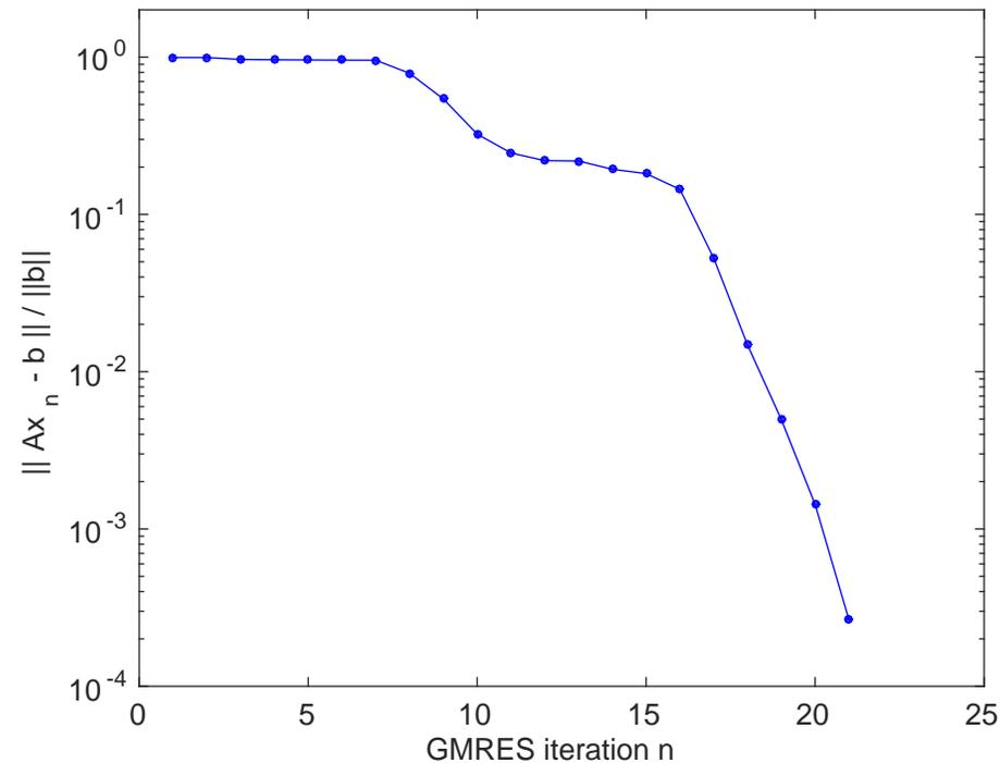
Computation of Newton step for periodic orbit of plane Couette flow
