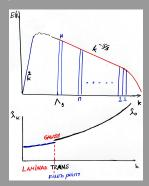
Figure: Schematic representation of scale elimination procedure and variation of dimensionless coupling constant  $\hat{\lambda}(k)$ . Re = Re(k).
