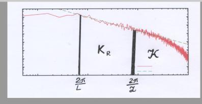
Figure: Length and energy scales in a flow. Dotted line:  $E(K) = C_{\mathcal{K}} \mathcal{E}^{\frac{2}{3}} k^{-\frac{5}{3}}$ .  $C_{\mathcal{K}} \approx 1.5 - 1.8$ .
