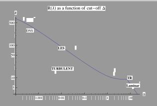
Figure: PROGRAM: study variation of the Reynolds number  $R_{\lambda}(\Delta)$  with the u.v. cut-off (filtering scale)  $\Delta$  in a turbulent flow with  $R_{\lambda,0} \approx 1000$  and the integral scale  $L = 2\pi/\Lambda_f \approx 10$ . By successive small-scale filtering we will derive formal expressions for DNS,LES and VLES.
