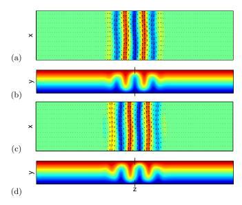
FIG. 1: (color online). Localized traveling wave  $\mathbf{u}_{\mathrm{TW}}$  (a,b) and equilibrium  $\mathbf{u}_{\mathrm{EQ}}$  (c,d) solutions of plane Couette flow at Re = 400, from [19]. The velocity fields are shown in the y=0 midplane in (a,c), with arrows indicating in-plane velocity and the color scale indicating streamwise velocity u: blue/green/red correspond to u=-1,0,+1. The x-averaged streamwise velocity is shown in (b,d), with y expanded by a factor of three.
